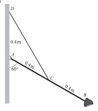
The diagram shows a wall-mounted light. It consists of a rod AB of mass 0.25 kg and length 0.8 m which is freely hinged to a vertical wall at A, and a lamp of mass 0.5 kg fixed at B. The system is held in equilibrium by a chain CD whose end C is attached to the midpoint of AB. The end D is fixed to the wall a distance 0.4 m vertically above A. The rod AB makes an angle of 60° with the downward vertical.
