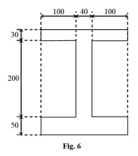
(i) Calculate the area of the beam's cross-section.
