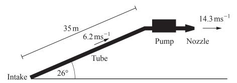
In order to model the changes to the mechanical energy of the chemical during the entire process of intake, drawing and discharge, the following modelling assumptions are made.
