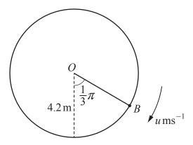
Given that the lowest speed of B in its motion is  $4 \,\mathrm{ms}^{-1}$  determine the value of u.
