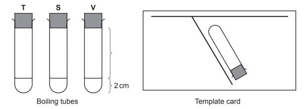
The students recorded the distance between the top of each liquid and the base of the rubber bung. They then tilted each tube to a 60° angle, using a template card for consistency, and measured the time taken for the first part of the liquid to flow down the tube and touch the rubber bung.
