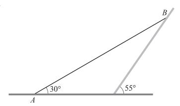
A uniform rod AB, of weight 20 N and length 2.8 m, rests in equilibrium with the end A in contact with rough horizontal ground and the end B resting against a smooth wall inclined at 55° to the horizontal. The rod, which rests in a vertical plane that is perpendicular to the wall, is inclined at 30° to the horizontal (see diagram).
