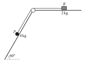
The diagram shows a small block B, of mass 2 kg, and a particle P, of mass 4 kg, which are attached to the ends of a light inextensible string. The string is taut and passes over a small smooth pulley fixed at the intersection of a horizontal surface and an inclined plane. The particle can move on the inclined plane, which is rough, and which makes an angle of  $60^{\circ}$  with the horizontal. The block can move on the horizontal surface, which is also rough.
