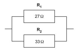
Calculate the total resistance of the resistor arrangement.
