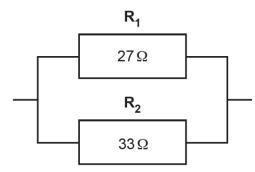
Calculate the total resistance of the resistor arrangement.
