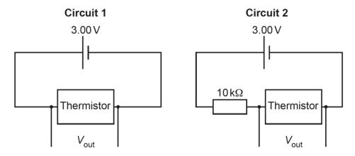
In each circuit, the voltage  $V_{\rm out}$  across the thermistor is connected to the heating system for warming the milk.
