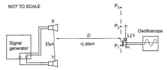
As the microphone is moved along the line  $P_1$  to  $P_3$  the oscilloscope shows maximum signal at  $P_1$ , zero signal at  $P_2$  and the next maximum signal at  $P_3$ .
