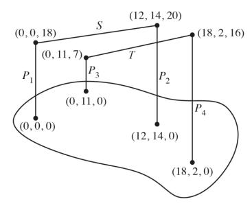
A vector equation of the line **segment** that represents the wire S is given by
