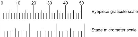
Stage micrometer scale
