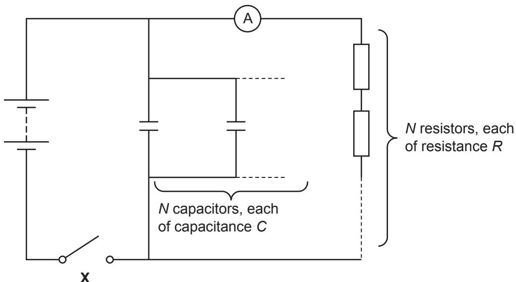
There are  $N$  capacitors, each of capacitance  $C$ , connected in parallel.
