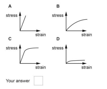
Candidates performed well on this question with most candidates correctly identifying graph A as most indicative of the stress-strain characteristics for a brittle material, as brittle materials exhibit minimal plastic deformation and the relationship between stress and strain is linear.
