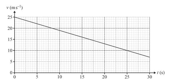
(a) A student argues that the speed of train A changes by  $18\,\mathrm{m\,s^{-1}}$  in 30 seconds so its acceleration is  $0.6\,\mathrm{m\,s^{-2}}$ .
