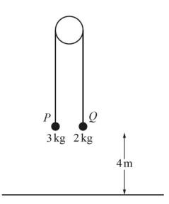
Two small balls P and Q, of masses 3 kg and 2 kg respectively, are attached to the ends of a light inextensible string. The string passes over a smooth fixed pulley. The balls are held at a height of 4 m above a horizontal floor, with the string taut. The parts of the string which are not in contact with the pulley are vertical (see diagram).
