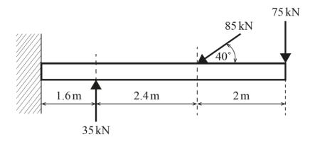
Calculate the vertical component of the 85 kN force.
