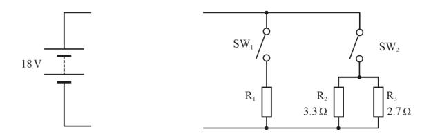
(a) Complete the circuit diagram so that current flows through the resistors when switches SW<sub>1</sub> and SW<sub>2</sub> are closed.
