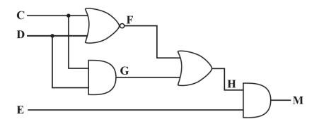
Complete the truth table for the logic circuit.
