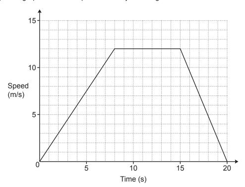
Calculate the distance travelled by the object during the 20 seconds.
