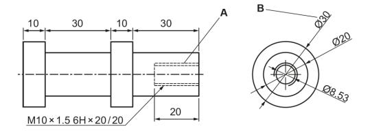
(a) State two mechanical features shown by label A.
