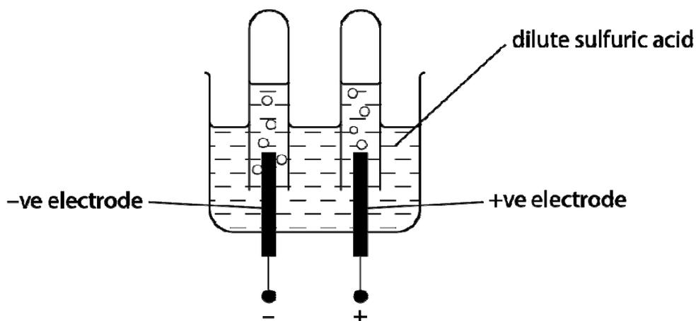
Hydrogen is made at the negative electrode.
