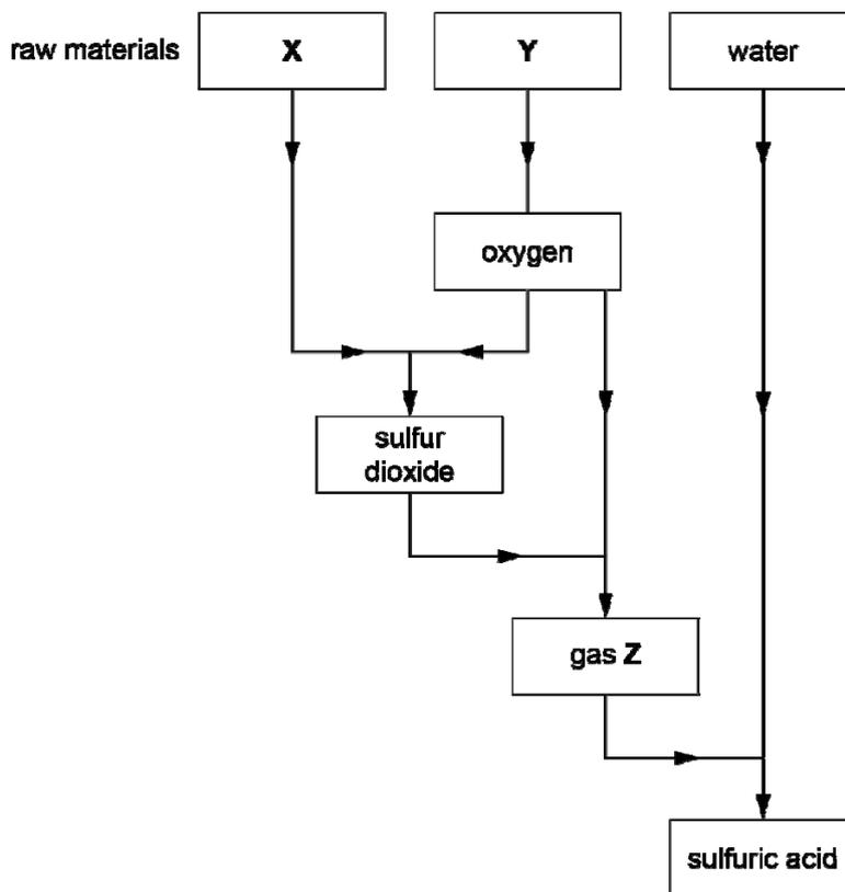
(a) The three raw materials used in the Contact Process are at the top of the chart.
