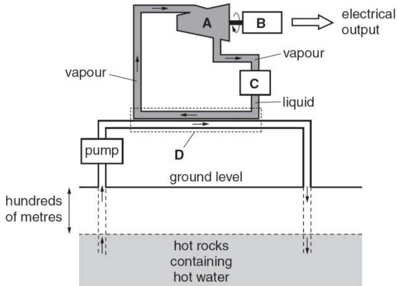
The four parts labelled **A**, **B**, **C** and **D** in the diagram are a condenser, a generator, a heat exchanger and a turbine.
