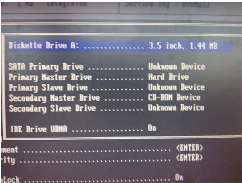
The HDD and CD-Rom Drive were both found. No other devices were connected, so there allocated slots appear as unknown.
